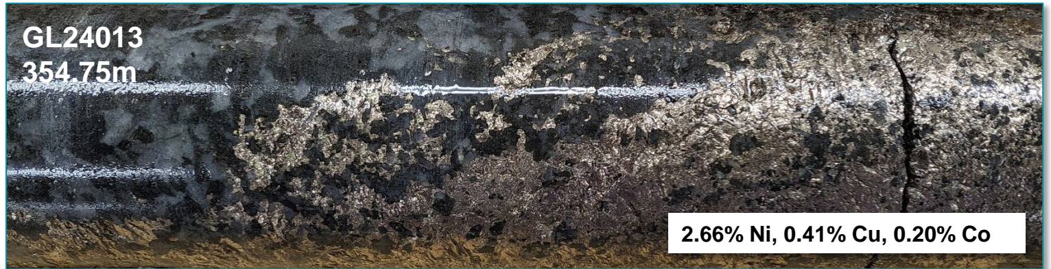
Breccia sulphide in contact with variable-texture gabbro
