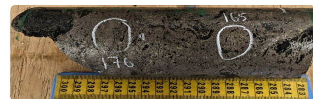
AL22051_108.99m; 2.13% Ni, 0.22% Cu, 1.73 g/t 3PE
