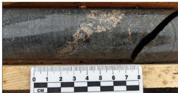
Gochager Lake: GL23010: 89.5m Medium grained gabbro with segregation of coarse-grained gabbro containing interstitial sulfide
