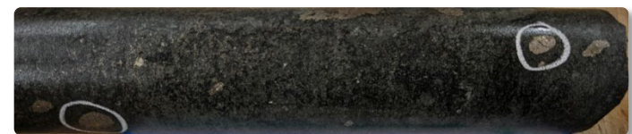
AL22040_120.80m; 0.44% Ni, 0.36% Cu, 0.31 g/t 3PE
