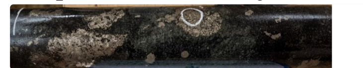
AL22040_121.14m; 0.41% Ni, 0.28% Cu, 0.32 g/t 3PE
