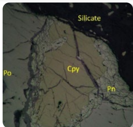
Polished Section of sulphide "globule" (AL22040); pentlandite (Pn) rimming chalcopyrite (Cpy)
